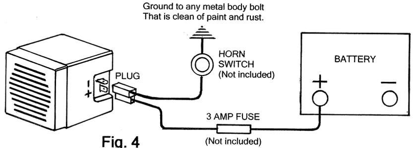
14. Connect the horn switch's other terminal to ground, any metal body surface that is clean of paint and rust.
