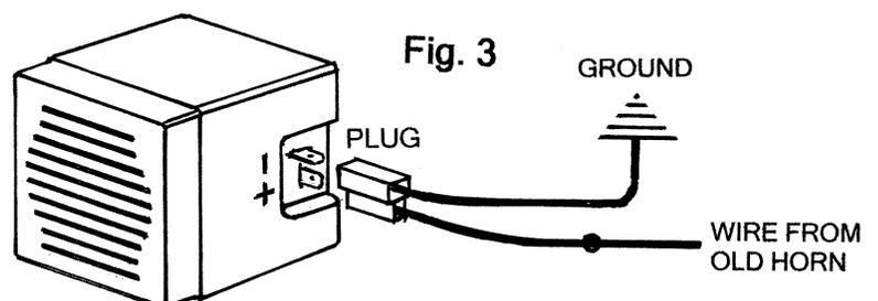
11. Connect the plug to the EE100. The horn installation is complete and the horn is ready to be used.
