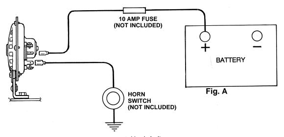
Ground to any metal body bolt that is clean of paint and rust.
