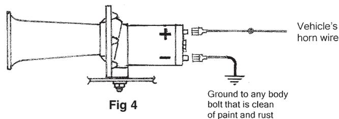
**IMPORTANT:** Always make sure that there is a 15-amp fuse is used in the horn circuit to protect the vehicle. When testing the horns, if the sound doesn't correct, reverse the wires connected to the terminals of the FUN HORN.
