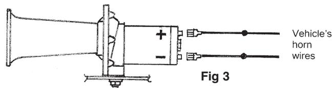
**IMPORTANT:** Always make sure that a 15-amp fuse is used in the horn circuit to protect the vehicle. When testing the horns, if the sound doesn't correct, reverse the wires connected to the terminals of the FUN HORN.
