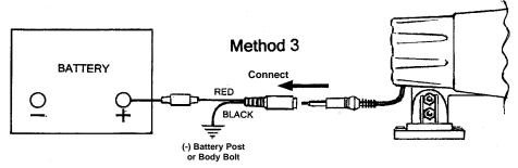
Red wire: is connected to a positive (+). Secure the red wire to the vehicle's battery, fuse-block or any covenant 12-volt (+) power source. Please note:to protect POWER PLAY and your vehicle there is an inline replaceable fuse,3-amp.
