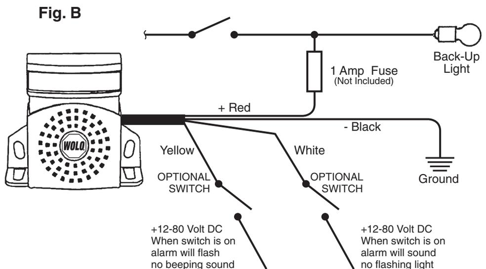
6. **IMPORTANT:** The back-up alarm must be wired as above steps 4 & 5. If the polarity is reversed, the alarms will not operate. This alarm must have a good connection to both power and ground to work reliably. Use 18-gauge wire (minimum) to lengthen wire leads if required. Make sure that all wires are secured and inspect to ensure that they will not interfere with vehicle's operation. Always make sure that any wiring is in accordance with the vehicle manufacturer's recommendations.
