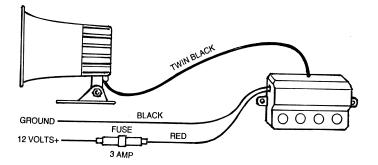
5. RED WIRE, is connected to the fuse-block or a under dash wire that has power (+) 12 volts when the ignition is on. **IMPORTANT:** To protect your horn and vehicle, use the inline fuse provided and wire as shown.
