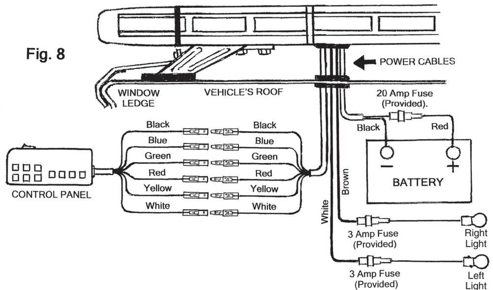
23. **RED WIRE:** Connect to positive (+) 12-volts such as the fuse block, accessory power source in the dashboard area or the positive (+) battery post. Always use the provided 10-amp inline fuse. Make sure the connection is at a location free from corrosion or oxidation.
